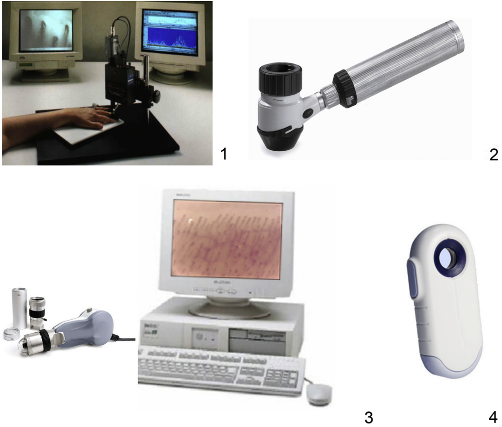
Fig. 3. Different devices for the capillaroscopic analysis. The widefield microscope (1). The dermatoscope (2). The video-capillaroscope (3). The ophthalmoscope (4).
